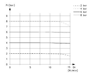
Pr = Outlet pressure (bar)\*  $Qn = Flow (NI/min)^*$
